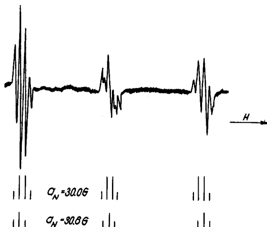
Fig. 1. The esr spectrum and the stick diagram of the two iminoxy radicals obtained from (II).
